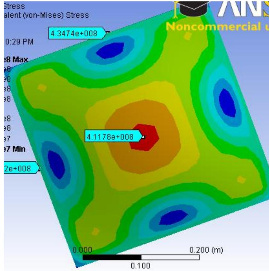
Finite element analysis of representative wall panel.
