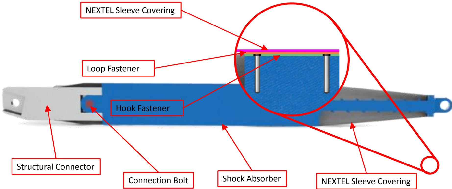
Cross section of shock absorber assembly, covered by NEXTEL sleeve
