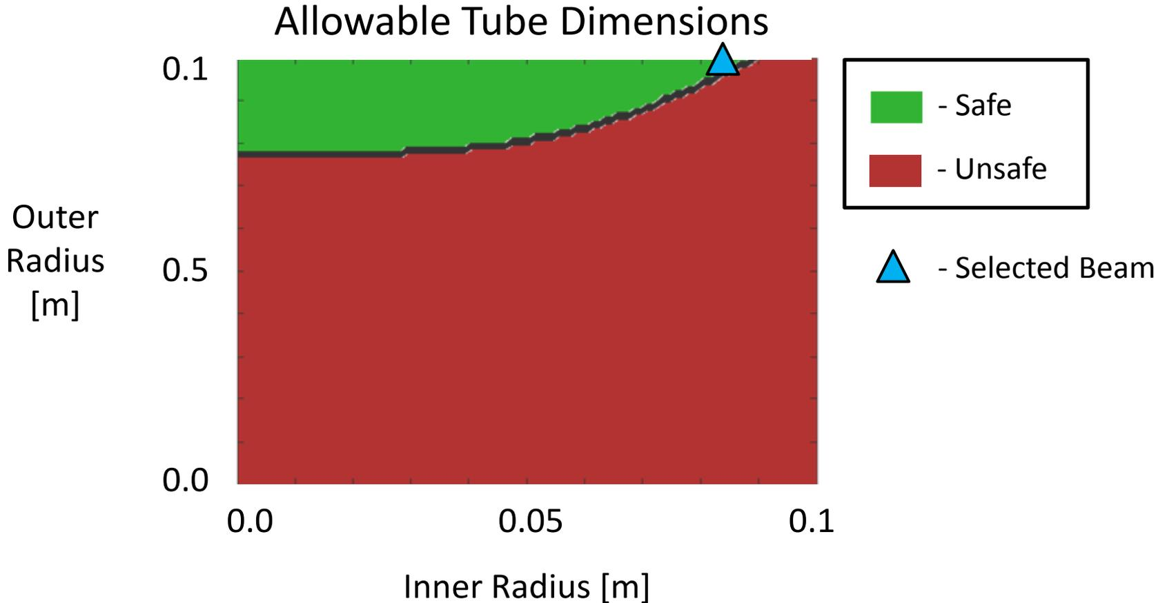
Analysis of critical tubular beam in compression; buckling and yield
