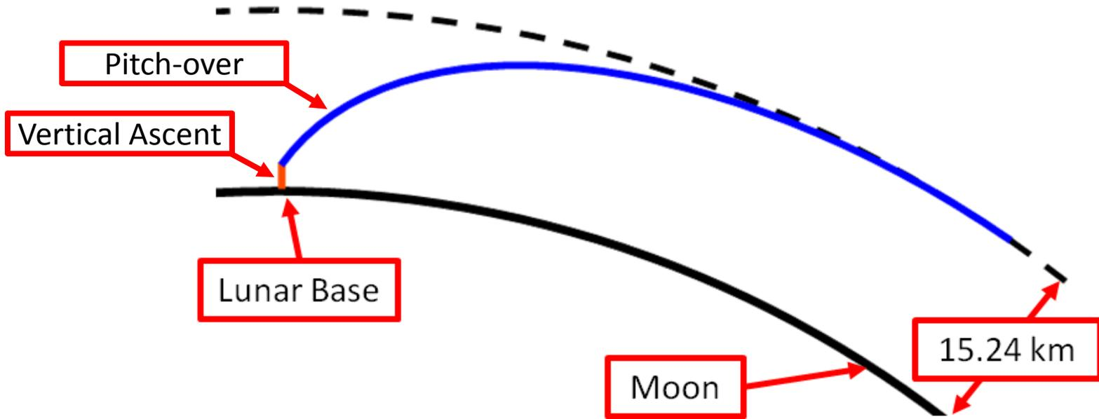
LEVITATE's trajectory from the lunar surface to orbit
