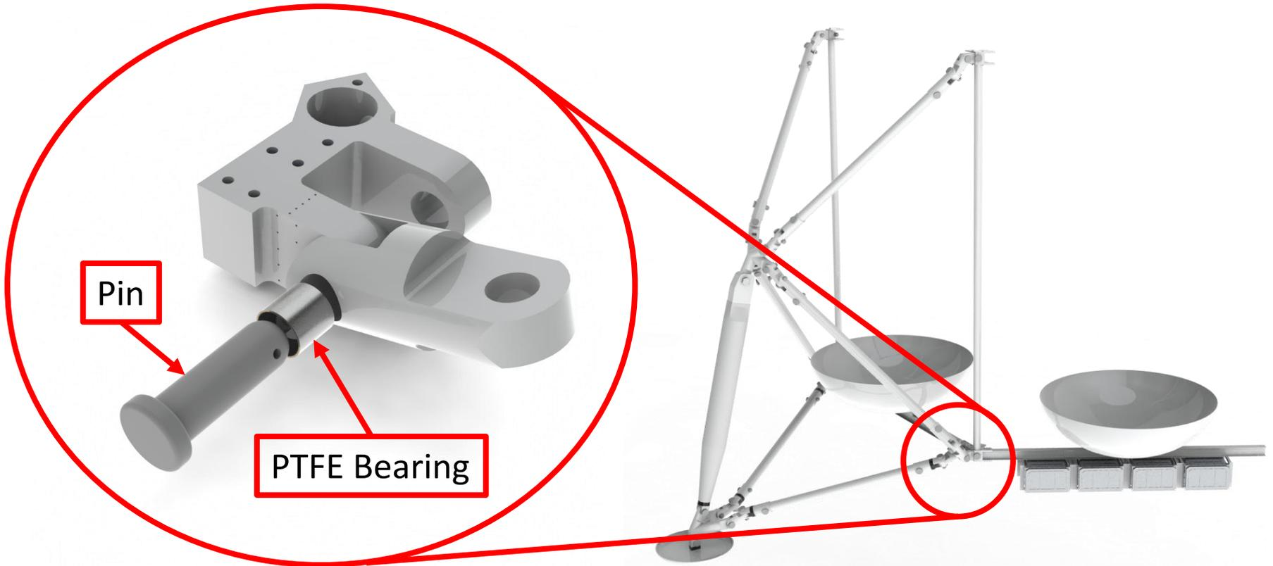
Exploded view of pinned connection showing pin, joint and bearing.
