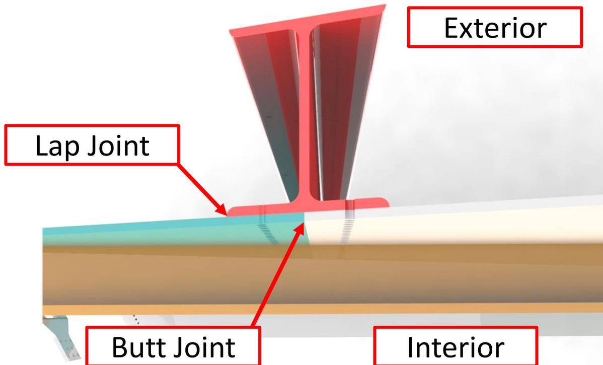
Wall panel section view showing I-beams and adjacent pressure panels
