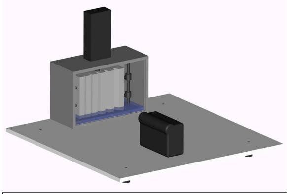
**Fig. 3-4** The experiment will be bolted to a <sup>1</sup>/<sub>4</sub>" thick aluminum plate which will be attached to our outer containment box with vibration damping neoprene sandwich mounts.
