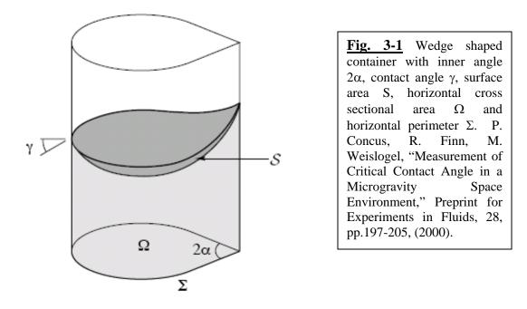
Another important property of the system is the fluid's contact angle with the container. This is an experimentally determined value which measures the angle at which the fluid contacts a material. A smaller contact angle indicates a stronger attraction between the fluid and the solid and therefore stronger capillary effects.
