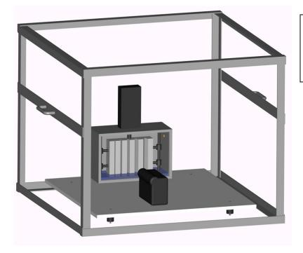
Fig. 3-3 Complete experimental assembly showing outer containment box and inner experiment
