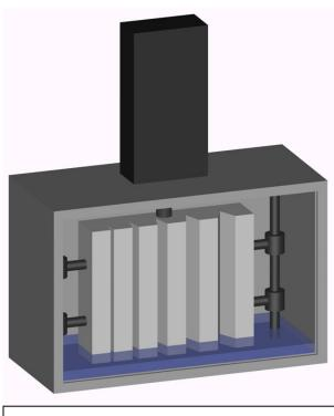
**Fig. 3-2** The fluid containment box containing the polycarbonate wedge piece with actuator mounted on top
