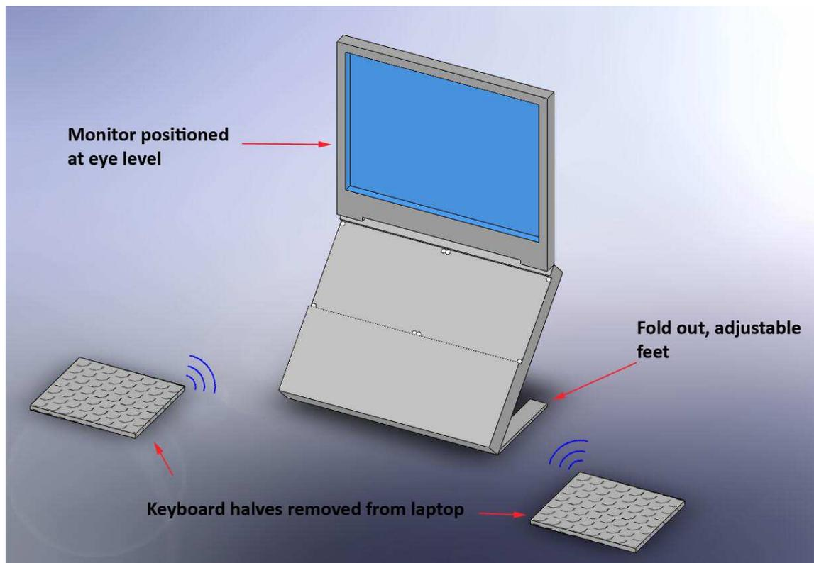
**Figure 4.** Removing the keyboard halves from the laptop and the addition of fold out braces allows the laptop to be positioned at the user's eye level for enhanced head and neck comfort in addition to the ergonomic benefits gained by separating and removing the keyboard halves.
