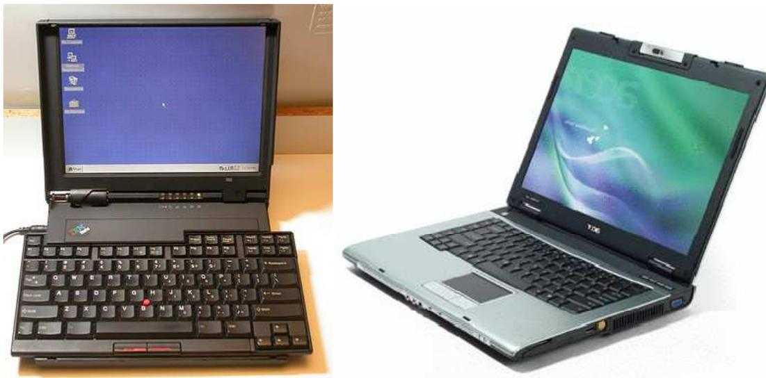
**Figure 2.** Left: The IBM ThinkPad 701C featured an expanding keyboard to provide full size keys. Right: Acer TravelMate 2482 with a gently curved keyboard.
