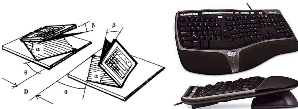
**Figure 1.** Left: Rotational axis definition; courtesy Marklin and Simoneau.<sup>11</sup> Right: Microsoft Natural Keyboard Elite 4000, exhibiting slant, gable, and slope key rotations.
