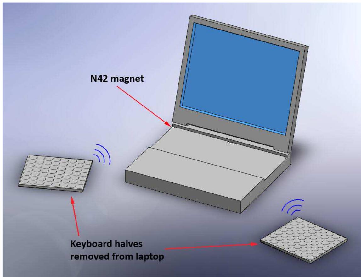
**Figure 3.** Initial wireless conception with keyboard halves removed from the computer. In the preferred conception, eight magnets embedded in the perimeter of the keyboard depression align with similar magnets mounted on the undersides of the keyboard halves. These magnets are oriented so that they are attracted to each other in order to effectively secure the keyboard while permitting easy, intentional removal.
