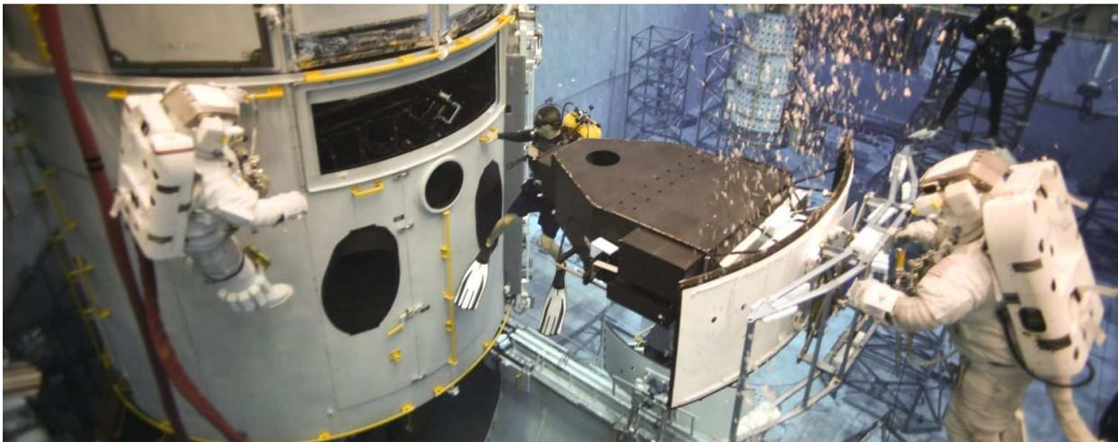
**Figure 3.** Practice installation of the Wide Field Camera 3 by Mission Specialists John Grunsfeld, left, and Andrew Feustel, right. Astronaut Feustel cannot see around the camera assembly, requiring Astronaut Grunsfeld to give him verbal directions as to the alignment and progress of the camera into the camera bay. Photo courtesy NASA.
