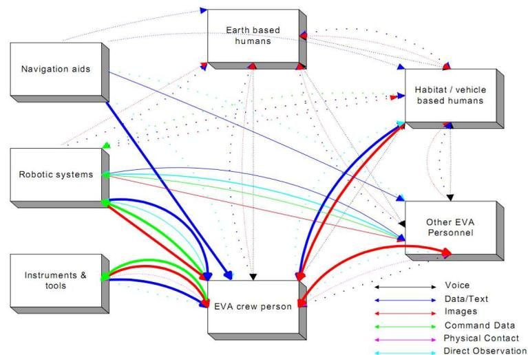
Figure 2. Communications web in support of extravehicular activities. Courtesy Boucher, et. al.<sup>8</sup>
