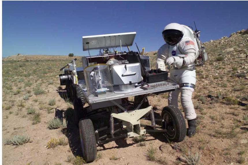
Figure 4. Prototype spacesuit and mobile experiment station.
