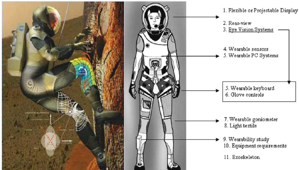
Figure 5. MIT's form-fitting unpressurized BioSuit concept. Courtesy Canina, Newman, and Totti.<sup>18</sup>
