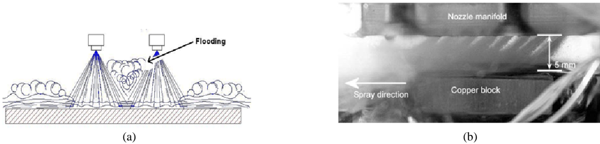
FIGURE 1. (a) Liquid flooding occurs in sprays directed perpendicular to the heated surface, impairing the formation of sprays (Glassman, 2005). (b) Spray configuration as used by Shedd on which the present experiment is based (2007). A hot surface ('copper block') is cooled by sprays angled at 45° to prevent the formation of a vapor dome on the surface and direct fluid towards the drain.
