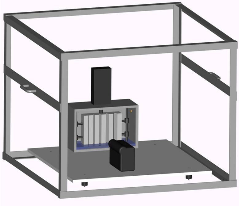
**Fig. 3-3** Complete experimental assembly showing outer containment box and inner experiment
