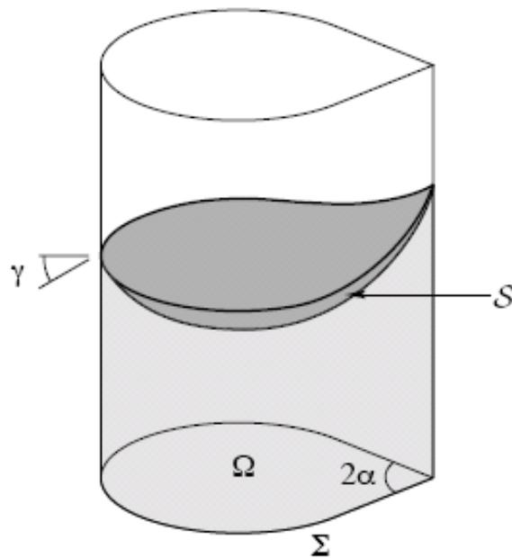
**Fig. 3-1** Wedge shaped container with inner angle  $2\alpha$ , contact angle  $\gamma$ , surface area  $S$ , horizontal cross sectional area  $\Omega$  and horizontal perimeter  $\Sigma$ . P. Concus, R. Finn, M. Weislogel, "Measurement of Critical Contact Angle in a Microgravity Space Environment," Preprint for Experiments in Fluids, 28, pp.197-205, (2000).
