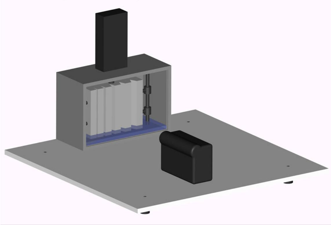
**Fig. 3-4** The experiment will be bolted to a 1/4" thick aluminum plate which will be attached to our outer containment box with vibration damping neoprene sandwich mounts.
