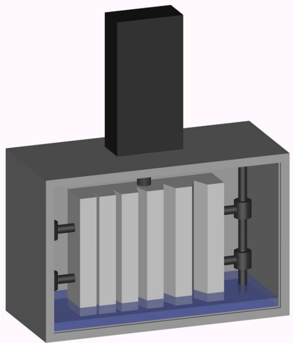
**Fig. 3-2** The fluid containment box containing the polycarbonate wedge piece with actuator mounted on top
